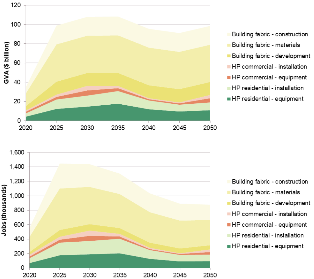
Figure 7. GVA and jobs directly supported by global deployment of heat pumps and building envelopes
